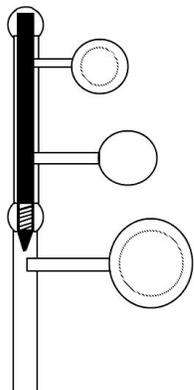
Improperly built hinge-pivot has worked loose but looks as if it is screwed in properly.
