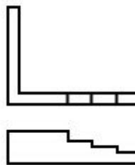
notice the three steps for measuring the proper key heights. The smallest is for the trill keys and the higher C key, the middle is for the rest of the main body keys and the third step is for the foot joint keys.
