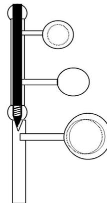
One other situation can cause the same problem but is more obvious. When a properly built hinge-pivot screw has worked its way loose the end of the hinge-pivot can be seen protruding from the top post.
